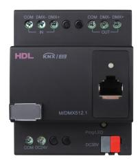
KNX/DMX recorder is not only a KNX/DMX gateway which supports two-way control, but also can make record, play back and delete DMX program from the ETS software or KNX wall panel .The maximum record time is up to 4 hours. This module can be used to control devices with built-in DMX protocol such as LED color changer, moving head ,laser light.
