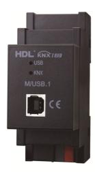
The M/USB.1 is a new KNX BUS interface with the USB connector galvanically is isolated from the KNX BUS that establishes a bidirectional date connection between PC and KNX BUS. The device enables addressing, setting parameters, visualization, protocoling and diagnosis of bus devices. The USB socket and bus connection is on the front of the device together with yellow LEDs. Each one is an indicator to show the status and traffic concerning the bus and the PC.
